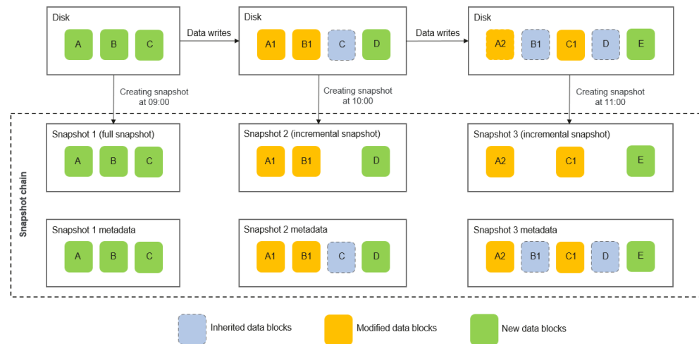
Figure 8-3 Snapshot chain with snapshots added
