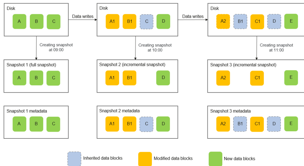
Figure 8-2 Standard snapshot principles
