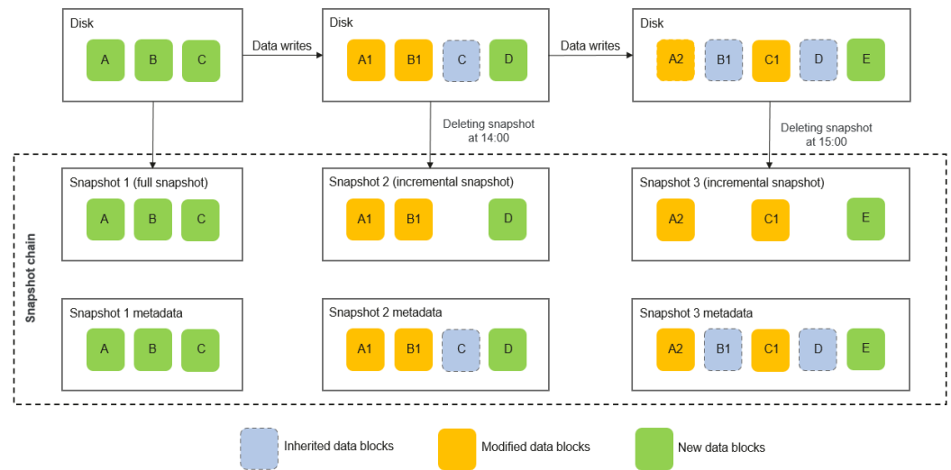
Figure 8-5 Snapshot chain with snapshots deleted
